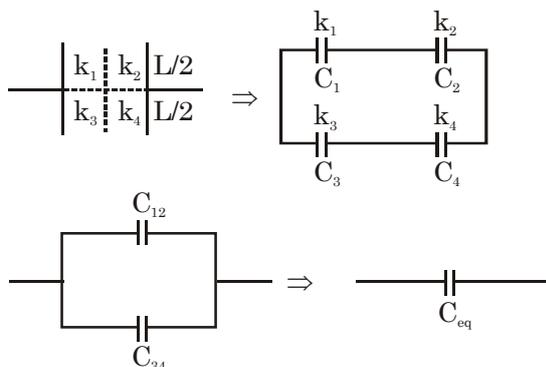
$$C_{12} = \frac{C_1 C_2}{C_1 + C_2} = \frac{k_1 \epsilon_0 \frac{L}{2} \times L}{d/2} \cdot \frac{k_2 \left[ \epsilon_0 \frac{L}{2} \times L \right]}{d/2}$$
