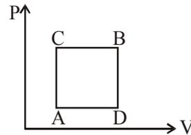
When path ACB is used 60 J of heat flows into the system and 30 J of work is done by the system. If path ADB is used work done by the system is 10 J. The heat flow into the system in path ADB is :
