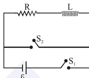
the switch  $S_1$  is closed at time  $t = 0$  and the switch  $S_2$  is kept open. At some later time ( $t_0$ ), the switch  $S_1$  is opened and  $S_2$  is closed. The behaviour of the current  $I$  as a function of time ' $t$ ' is given by :
