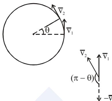
$$\begin{aligned} |\Delta \vec{v}| &= \sqrt{v_1^2 + v_2^2 + 2v_1v_2 \cos(\pi - \theta)} \\ &= 2v \sin \frac{\theta}{2} \quad \text{since } [|\vec{v}_1| = |\vec{v}_2|] \\ &= (2 \times 10) \times \sin(30^\circ) \\ &= 10 \text{ m/s} \end{aligned}$$
