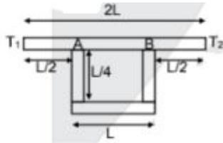
If temperature difference  $T_1 - T_2$  is  $120^\circ\text{C}$ . The temperature difference between points A & B is
