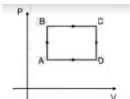
For path ABC, Heat given to the system is 60 J and work done by the system is 30 J.
